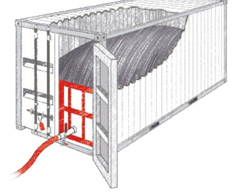
Flexitanks have a capacity of 16 to 24 cubic metres and are particularly well-suited for transporting liquid non-hazardous chemicals and foodstuffs.
